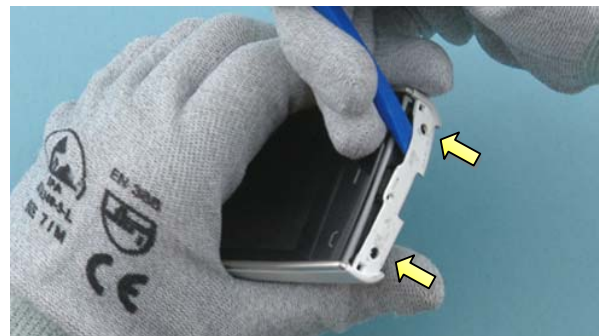
10) Release the clips on the bottom side of the device with the SS-93.
