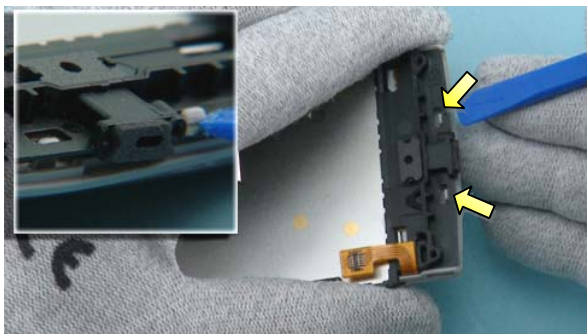
33) Release the two clips holding the UI-KEYMAT ASSY using the SS-93.
