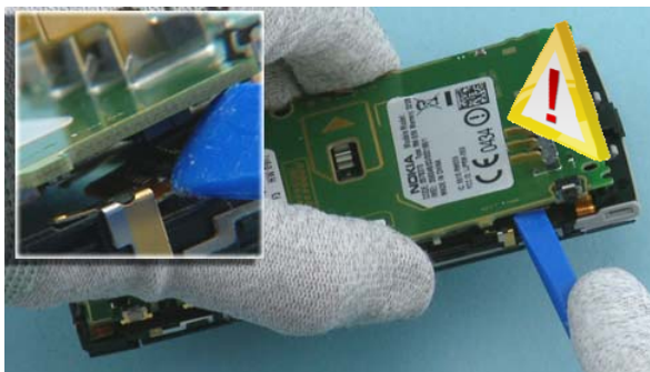
23) Disconnect the UI FLEX with the SS-93. Be careful not to damage the connector or nearby components!
