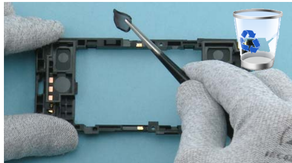
22) Remove the IHF TAPE with the tweezers. Do not use it again.
