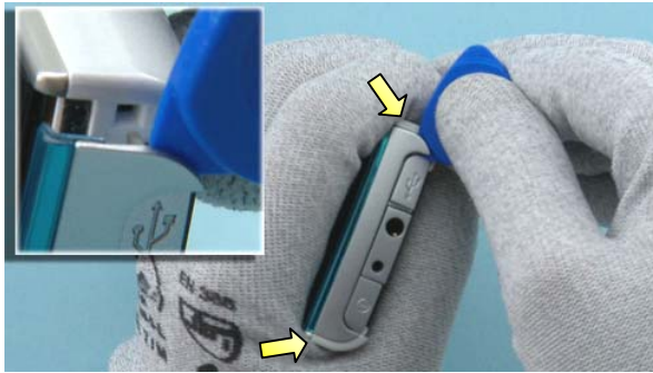
7) Use the SRT-6 to release the clips and the adhesive holding the TOP COVER ASSY.
