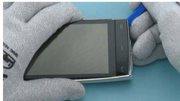
12) Release the SIDE COVER ASSY on bottom side as shown.
